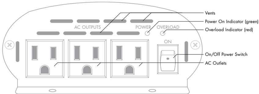
**ON/OFF Switch** – Controls operation of the inverter. The below indicators operate when the switch is ON.
