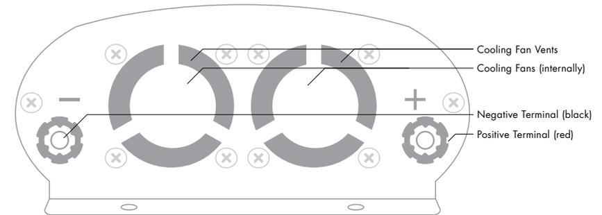
**High Speed Fan** – Keeps the inverter circuitry cool. The fan operates when the inverter is powered on. To avoid unnecessarily draining of the battery, turn off the inverter when it is not in use.
