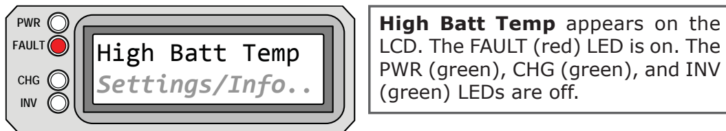
Figure 5-23, High Battery Temperature Fault
