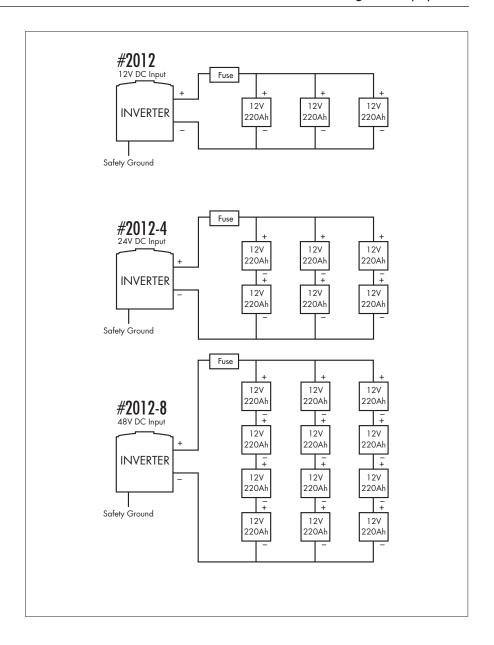
WARNING: EXPLODING BATTERIES CAN SPRAY MOLTEN LEAD, HOT SULFURIC ACID AND PLASTIC FRAGMENTS. BATTERIES THAT ARE CHARGING OR UNDER HIGH DISCHARGE RATES CAN PRODUCE EXPLOSIVE HYDROGEN GAS INTO THE SURROUNDING AREA. BE SAFE—FUSE THE BATTERY BANK AND MAKE SURE THE BATTERY BANK LOCATION IS PROPERLY VENTILATED.
