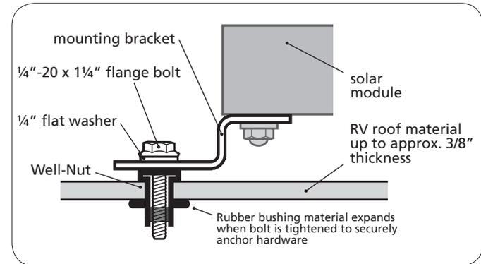
Fig. 8. Attaching 5-hole mounting bracket to RV roof
